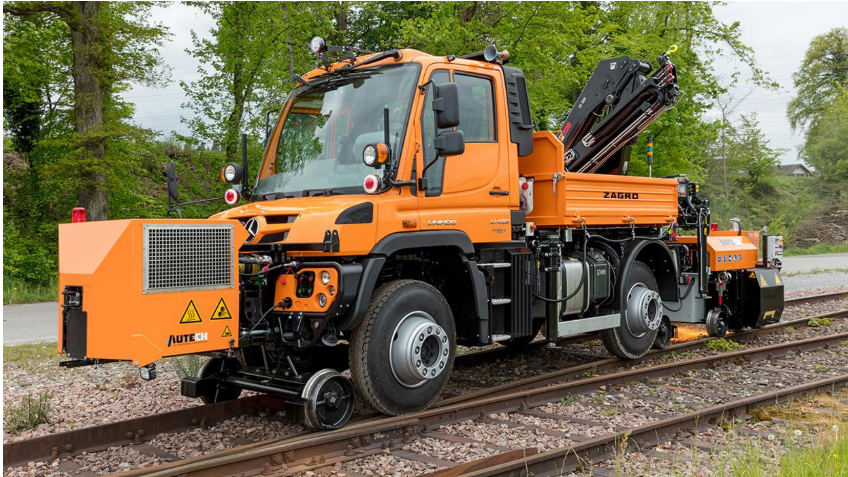
9 identical vehicles for MÁV (Hungarian State Railway) with swap bodies (here: crane and grinding unit)
